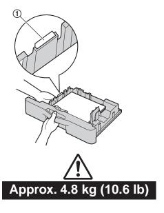
Do not position the unit in a location where it is unstable or subject to vibrations. The unit weighs approximately 35 kg (77 lb) when the lower input tray is installed and fully loaded with recording paper.
